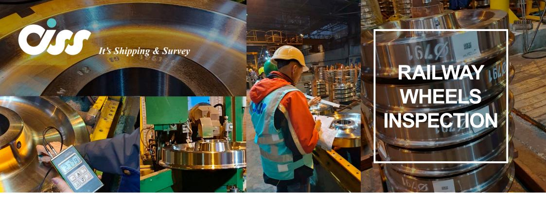
Wheels are cast or forged and are heat-treated to have a specific hardness. New wheels are trued, using a lathe, to a specific profile before being pressed onto an axle. All wheel profiles need to be periodically monitored by **CISS GROUP**'s inspectors to ensure proper wheel-rail interface. Improperly trued wheels increase rolling resistance, reduce energy efficiency and may create unsafe operation.
