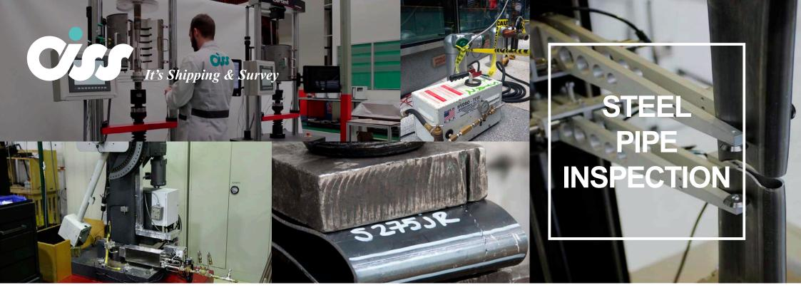
The mechanical Destructive and non-destructive tests are types of pipe inspection which confirms the mechanical requirements of pipe are as per the material standard. The tensile test is done to check the yield and ultimate tensile of the pipe. If required by the purchaser or by standard high or lowtemperature tensile tests are also performed.
