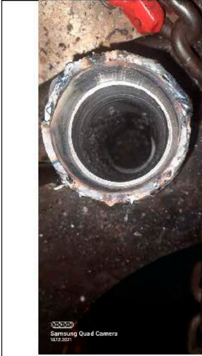
Welded additional pipe to make a wrench lever
